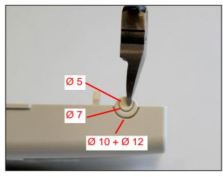
Fig. 5 Cutting the required opening dimension (cover)
