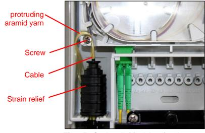
Fig. 15 Strain relief for inlets / outlets
