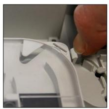
Fig. 12 Pull back the snap-in hook to open the cassette
