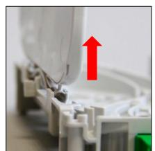
Fig. 13 (Prior to population) Remove cassette upward
