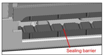
**Fig. 18d** Sealing insert for 12x LC plug, Ø 2 mm
