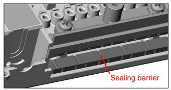
Fig. 18c Sealing insert for 6x SC plug, Ø 2 mm
