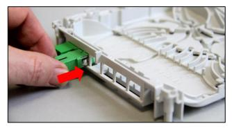
Fig. 11b Inserting the coupling
