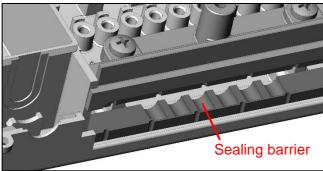
**Fig. 18a** Sealing insert for 6x cable, Ø approx. 7 mm
