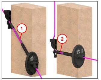
The system can be installed straight at 90° (2) or inclined (1) up to 45° upwards. Installation is identical in both cases.
