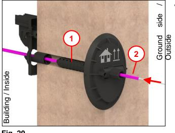
Pull the media cable (2) straight and • insert it through the foam pipe (1) from the ground side.
