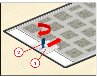
• Push back the locking flap (1) and lock it with the key provided (2) (clockwise).
