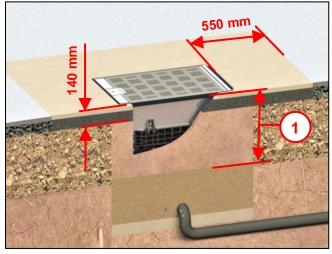
Construct the top layer (1) as per ZTV A-StB 12 (and/or Guidelines for the standardisation of traffic area top layers RStO 2001). In the vehicle traffic area: At the upper edge of the top layer, allow a strip of concrete or poured asphalt at least 550 mm wide and 140 mm thick (asphalt base layer of at least construction class V according to RStO 2001).
