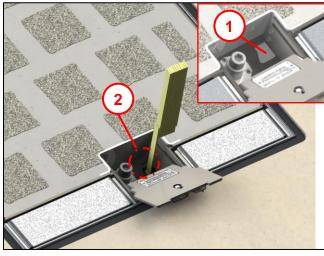
Opening to check the water level, e.g. in the event of flooding **(1)**. Doubles as a pump-out opening.
