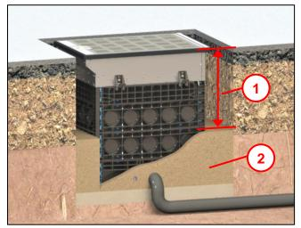
Backfill the foundation pit in layers using material suitable for compacting (2) in accordance with ZTV E-StB 09 up to the lower edge of the top layer (1). (Top layer height approx. 65 cm).
