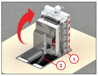
• Open the swivel cover until the safety catch (1) on the side engages.
