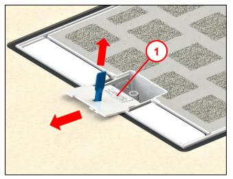
• Fold the locking flap (1) upwards and pull it forwards.
