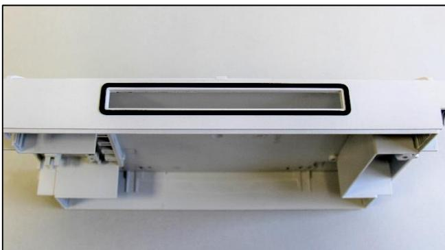
**Fig. 29** Inserting the seal
