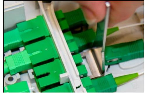
**Fig. 31** Coupling releas (not included in the delivery contents).
